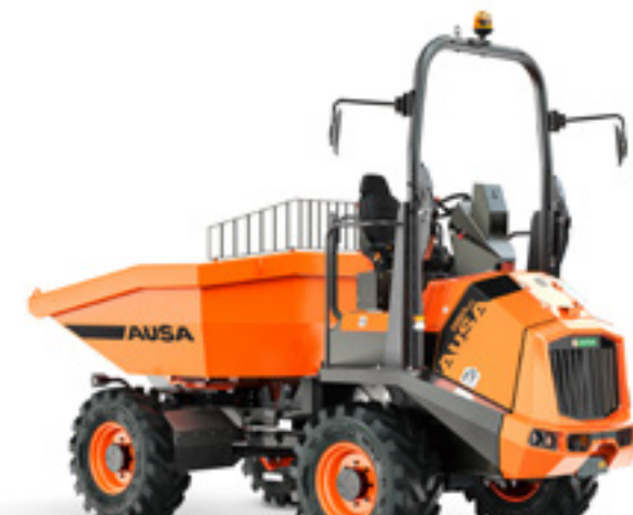
DR601AHG 13,200 lb UNLOADING SYSTEM ROTATING POWER 74.3 hp WIDTH 87 in TRANSMISSION HYDROSTATIC
