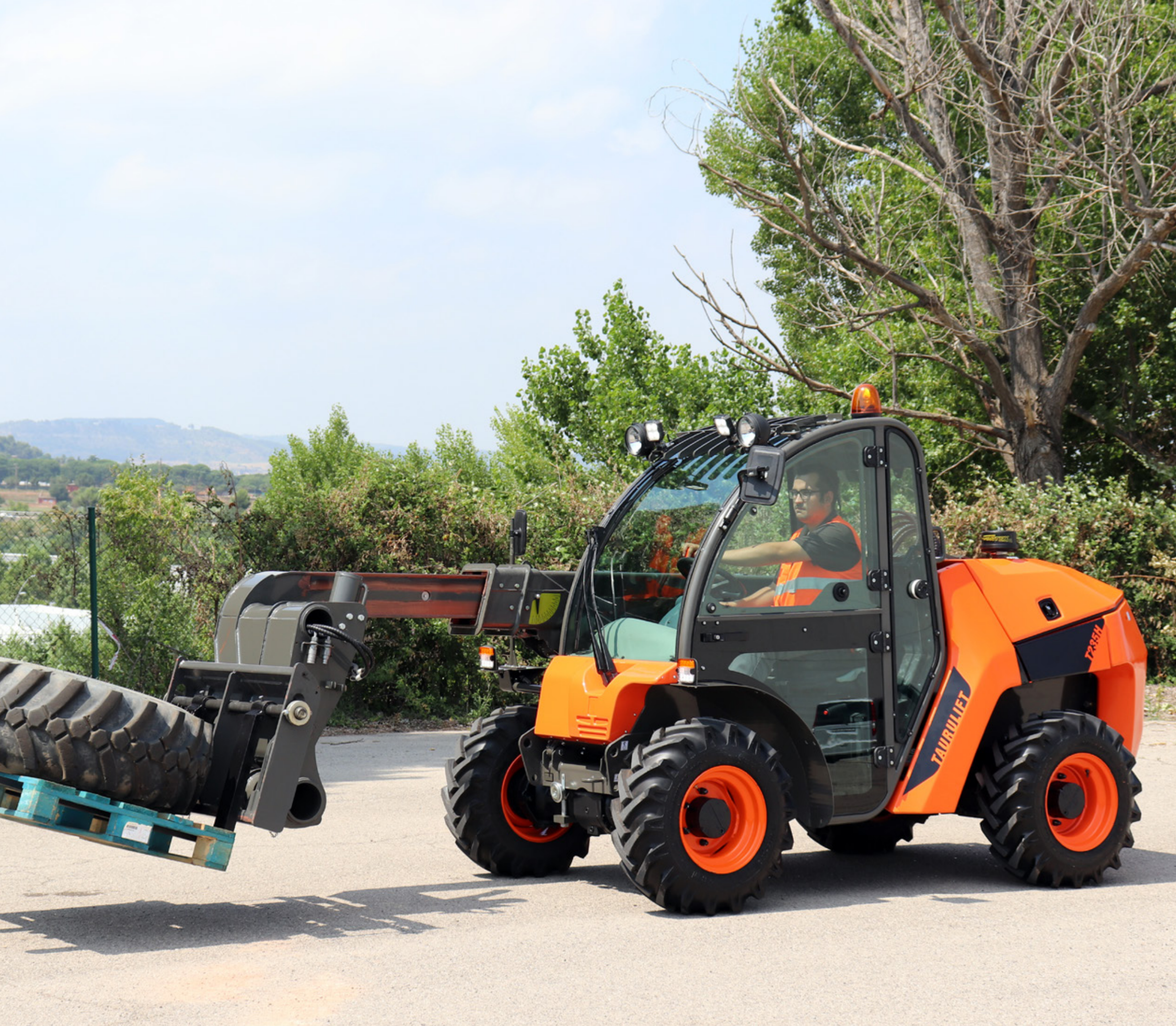
T204H 4,400 lb MAXIMUM LIFT 13.8 ft POWER 44.5 hp WIDTH 62.6 in TRANSMISSION HYDROSTATIC
