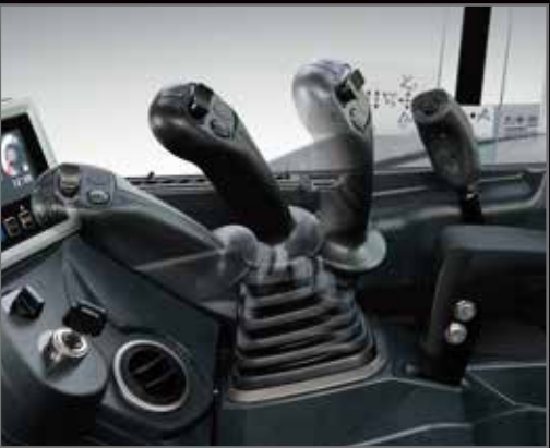
Ergonomic Lever Angles Operators can move levers horizontally without twisting their wrists, reducing fatigue.
