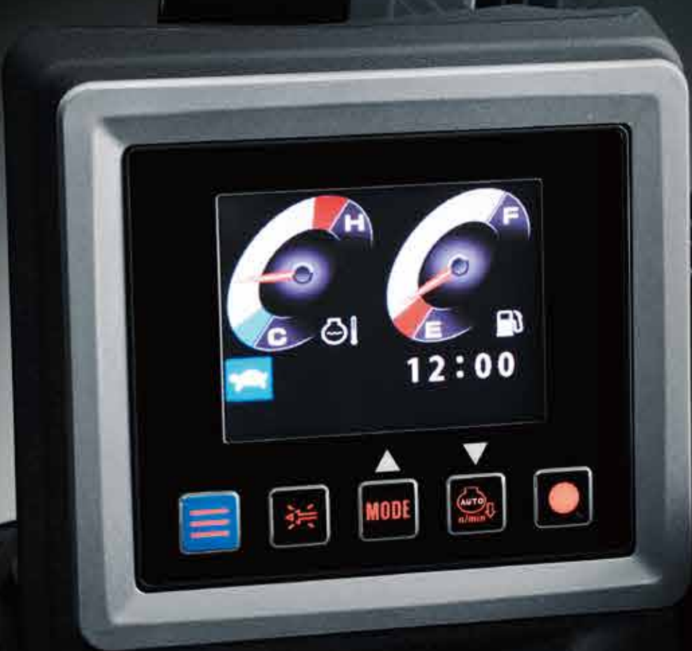
Color Monitor The new color monitor shows current and historical operating information in a clear and easy-to-operate format.
