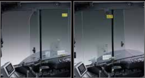
Slide-Open Window The right side window can slide open from the front or the back for increased ventilation and to hear ground workers when required.
