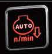
Auto Deceleration Auto deceleration saves fuel and lowers engine noise by lowering engine speed to idle.
