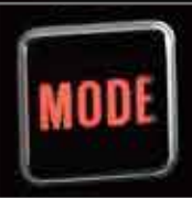
Energy Conservation Mode The SK45SRX/SK55SRX has 2 working modes, one for maximum power and S-mode for increased fuel economy.
