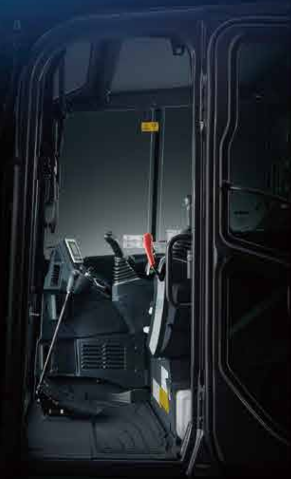
Ergonomic Lever Angles Operators can move levers horizontally without twisting their wrists, reducing fatigue.
