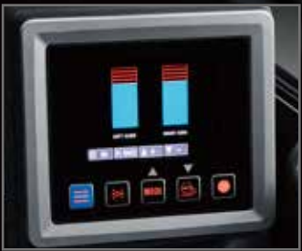
Auxiliary Hydraulic Flow Nibbler/breaker and rotation hydraulic flow has 6 presets that can be adjusted to match your attachment.
