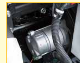
Starter motor Generator
