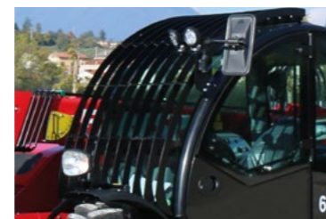
Front window protection grille.
