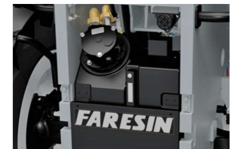
Hydraulic oil reservoir with oil level indicator.
