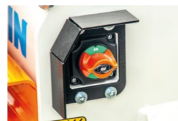
Manual battery switch, located on the front of the machine.
