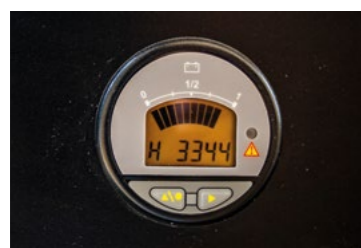
Battery monitoring system, positioned in its front part.
