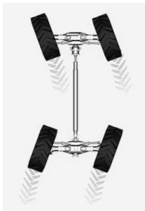
Concentric: guarantees a narrower manoeuvring radius.
