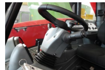
Adjustable steering column, via side lever.
