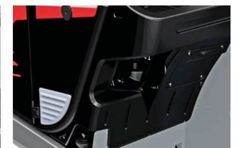
For engines with SCR, the Adblue tank is positioned at the rear.
