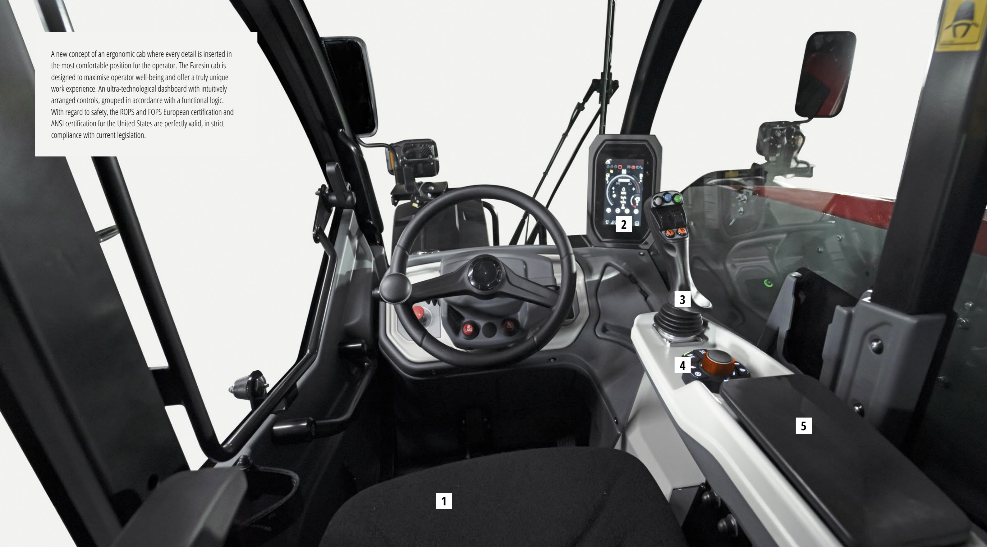
1 AIR SUSPENSION SEAT WITH MULTI-REGULATION TO REDUCE FATIGUE
