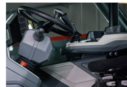
Steering column tiltable via side lever.
