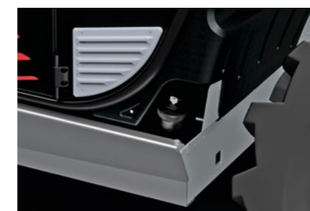
Fuel tank positioned under the cab for excellent protection (standard version).
