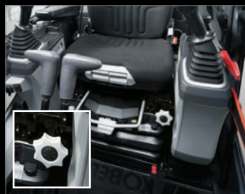
Adjustable height pilot valves
