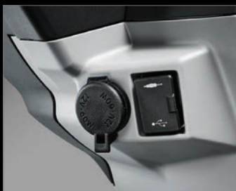
USB charging port / 12 V power socket
