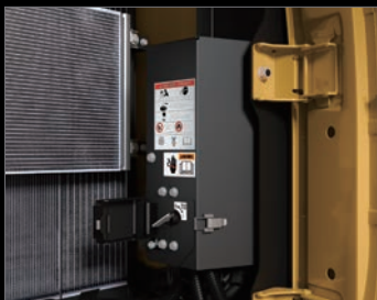
Battery Disconnect Switch with DEF Purge Notification Light
