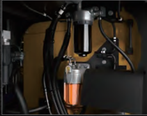
Fuel Filter / Pre-Filter with Integrated Water Separator
