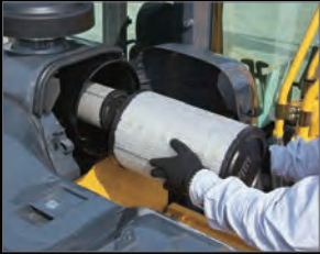
Two-Stage Air Filter
