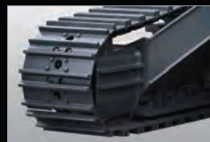
3 Heavy duty shoe (700 mm double bar grouser)
