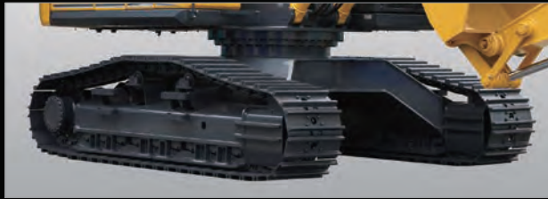
Overall width of crawlers 11'8" (3,550 mm)
