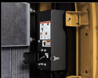
Battery Disconnect Switch with DEF Purge Notification Buzzer
