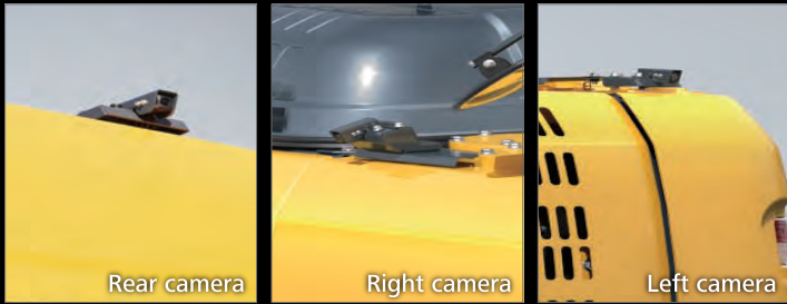
Standard Rear, Left and Right Side Cameras
