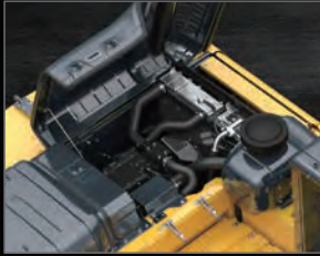
Engine Maintenance Lower service platform makes engine service easier.
