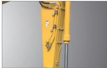
Quick coupler piping
