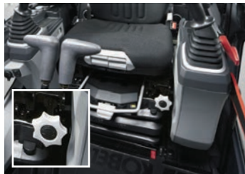
Adjustable height pilot valves
