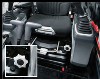
Adjustable height pilot valves
