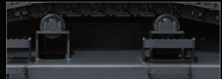
2 Large, double-support, outer flanged upper rollers
